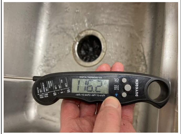
Windows within 24" of doors are to be safety glazing. Potable water temperature good just below 120F
